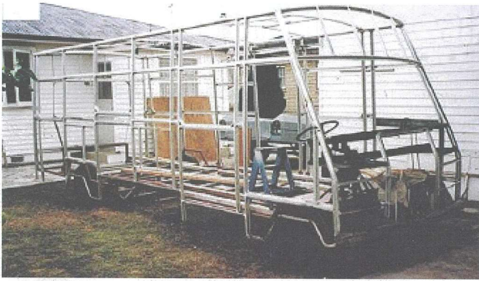
The 4 corner uprights and around the top edge were 2¼" diameter aluminium tube. The rest of the frame was 60 x 30 top hat aluminium section. This was all TIG welded.
